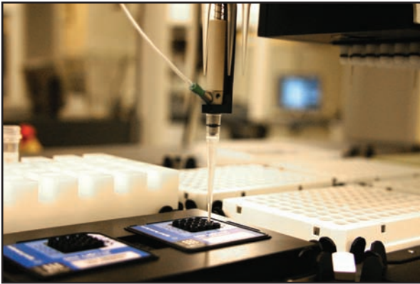
Figure 2. Sciclone ALH 3000 accessing a well on a LabChip
